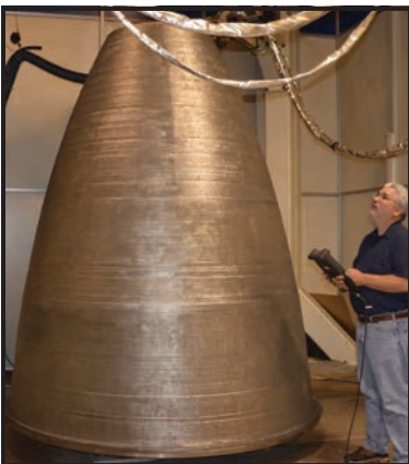
Figure 7. Full scale RS 25 rocket engine nozzle printed in multi-nozzle DMD system
