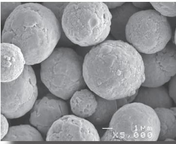
Spherical Conductive Nickel Powder
